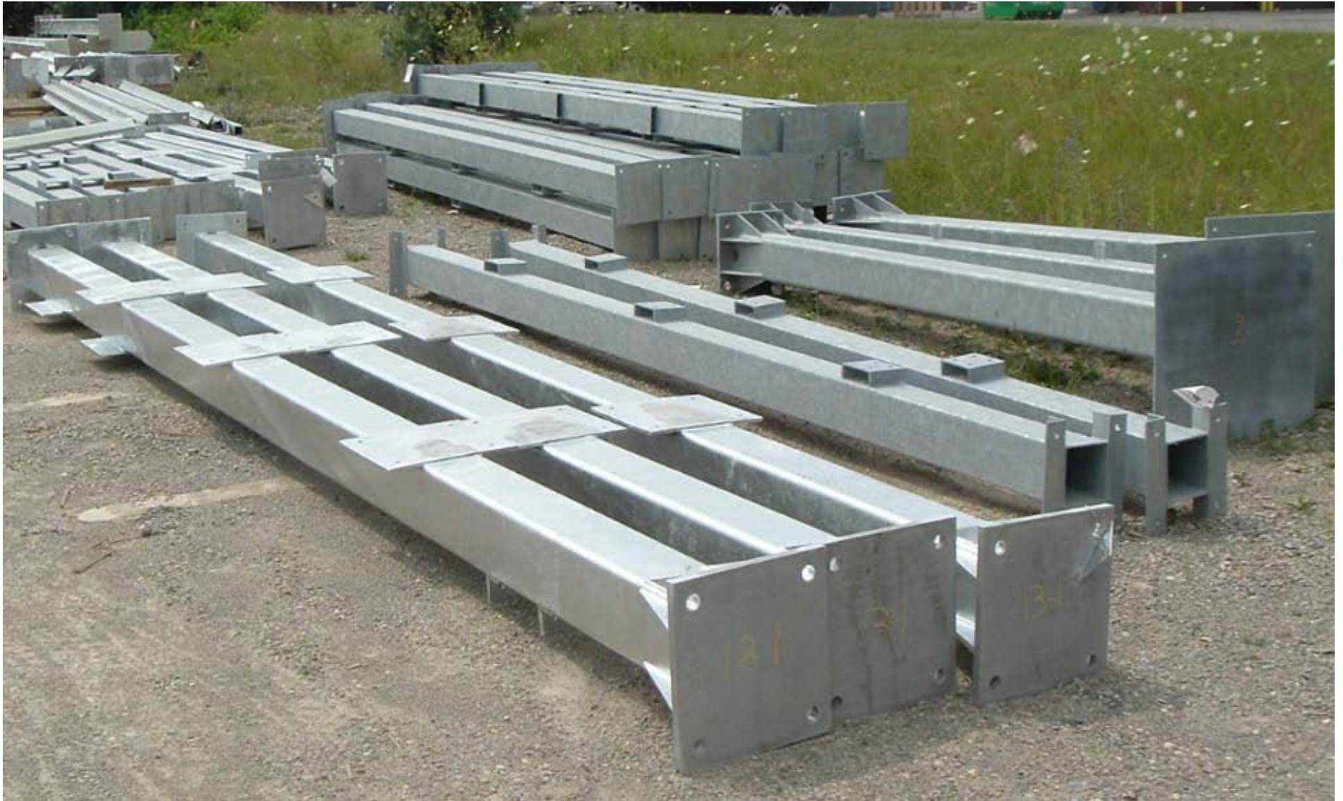
Galvanized HSS columns, beams and equipment stands ready for shipment to the jobsite. Note mark numbers painted on the end plates so they are covered after installation.
