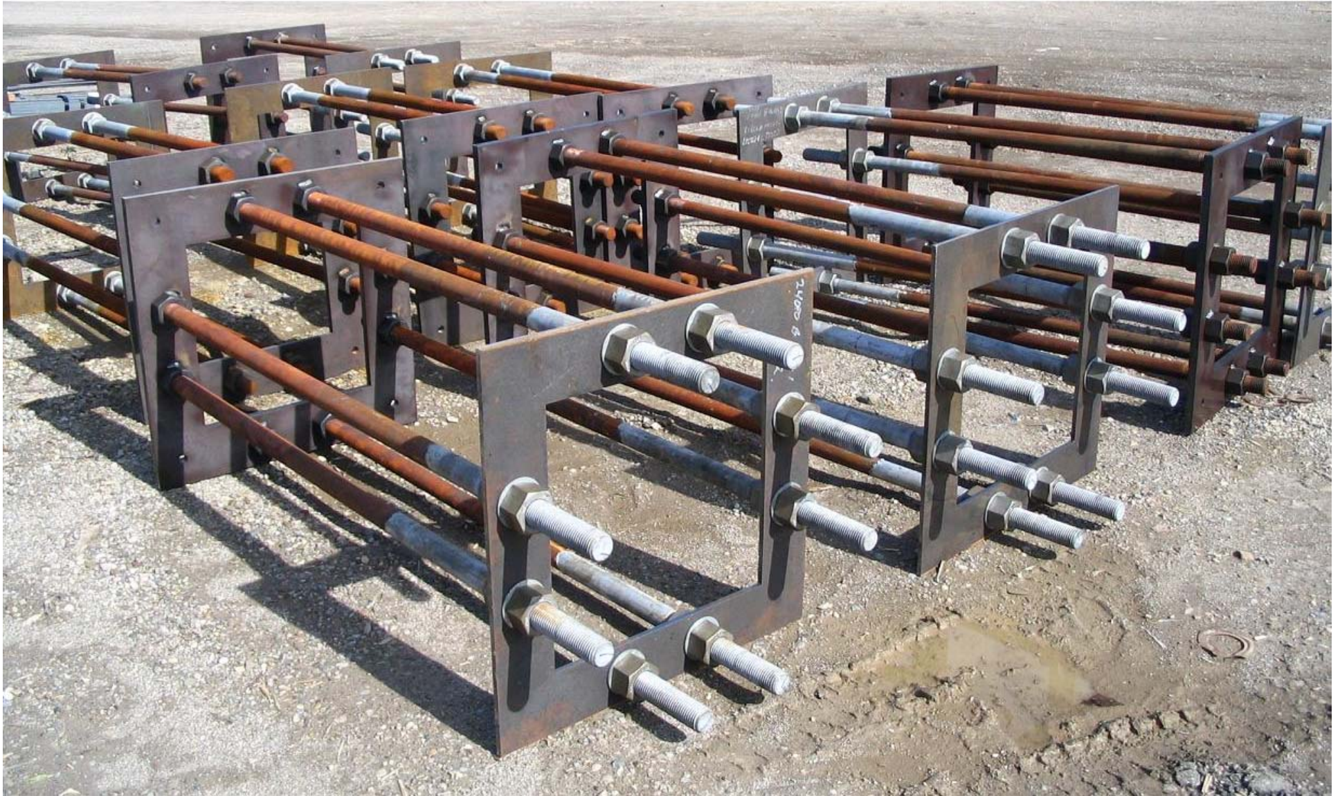
Anchor cages with partial galvanizing are assembled and ready for shipment.
