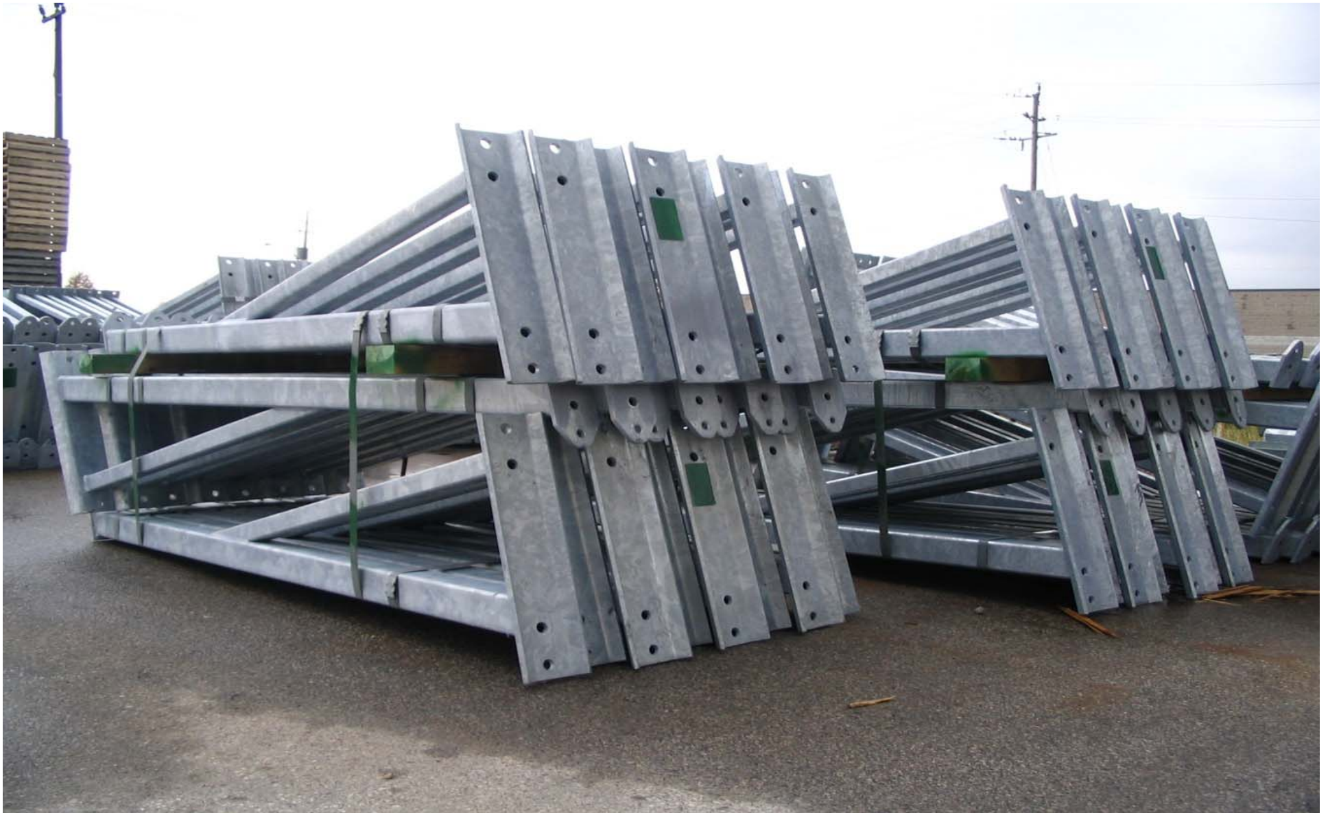
Suspension arms banded and colour coded for shipment to the Victor Mine 115 KV Transmission Line
