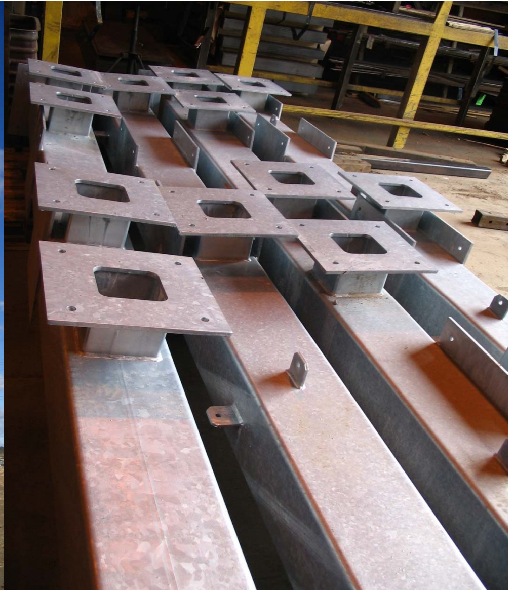
Columns showing beam connections stubs and grounding tabs.
